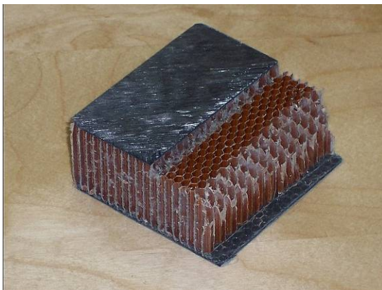
Cutaway of a test sample similar to a bulkhead showing Nomex sandwiched between layers of prepreg carbon fiber.
