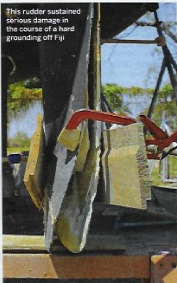
This rudder sustained serious damage in the course of a hard grounding off Fiji
